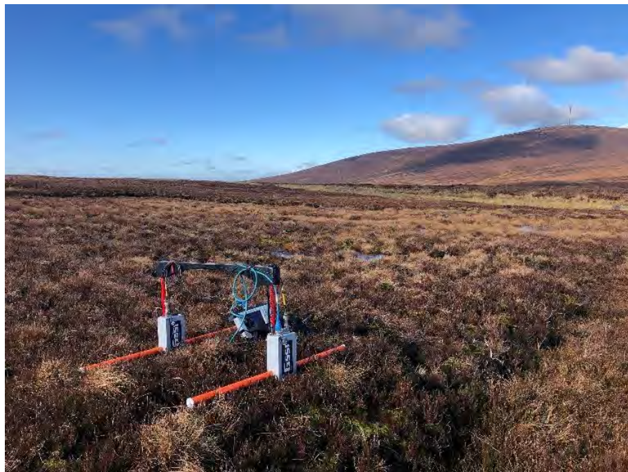
Figure 1: 80MHz GPR antenna operated from GSSI SIR 3000 system. Liffey Head Bog
